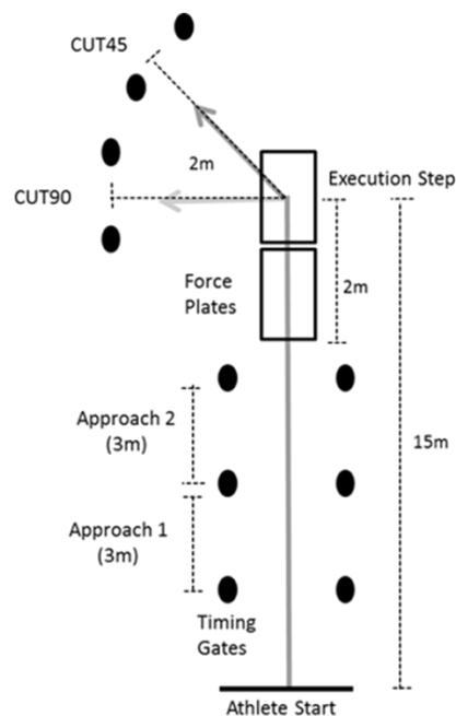
**Figure 3: Experimental setup for the cutting task. Solid line arrow represents line of motion with two cutting angles at the end. The light timer was triggered from 8m before force plate, and again 5m before the force plate.**
