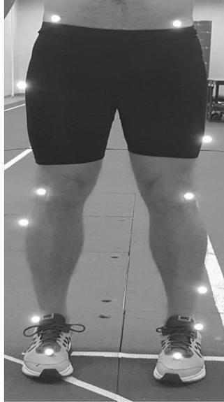
**Figure 2: Subject positioned for standing calibration trial with retro-reflective marker placed at relevant sites (heel and PSIS are posteriorly positioned). This is to establish local coordinate system relative to global that is marked via static and dynamic calibration with the wand.**
