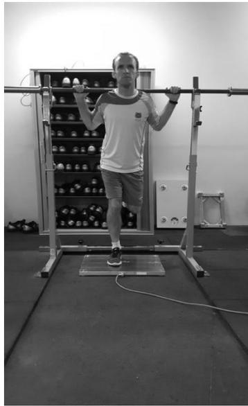
**Figure 1: Adopted subject positioning for the unilateral isometric strength test. Squat rack was bolted to the floor, and had custom made stoppers connecting the barbell to the rack.**
