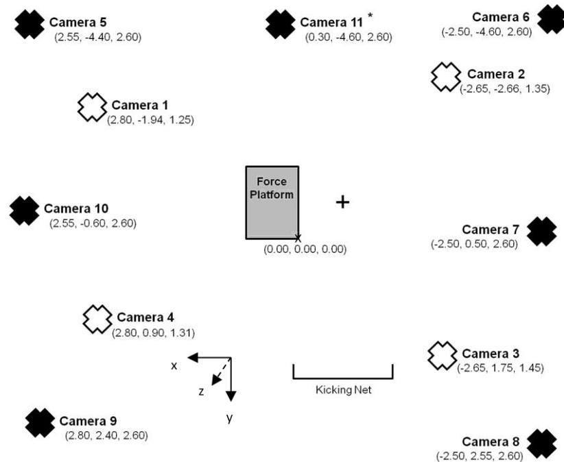
**Figure 4.2.** Camera setup for left-footed kickers (not to scale; all measurements taken from the corner of the force platform using an  $(x,y,z)$  coordinate system). \* denotes a camera only used in the 11 camera setup. (Cameras mounted on a rig suspended from the ceiling are marked with a black cross, cameras mounted on a tripod are marked with a white cross).
