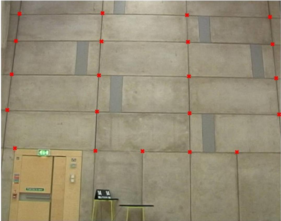
**Figure 3.2** The 21 calibration points measured and digitised to calibrate the ‘front’ camera to reconstruct the final 2D ball position (calibration dimensions at their widest point of 4.61 m × 9.06 m).
