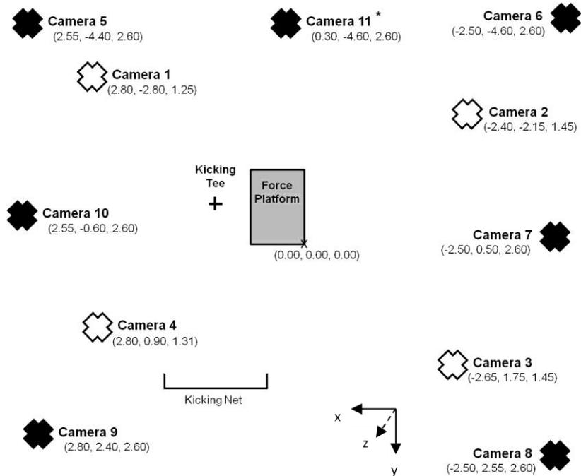
**Figure 4.1.** Camera setup for right-footed kickers (not to scale; all measurements taken from the corner of the force platform using an (x,y,z) coordinate system). \* denotes a camera only used in the 11 camera setup. (Cameras mounted on a rig suspended from the ceiling are marked with a black cross, cameras mounted on a tripod are marked with a white cross).
