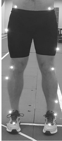
Figure 3: Subject positioned for standing calibration trial with retro-reflective marker placed at relevant sites (heel and PSIS are posteriorly positioned). This is to establish local coordinate system relative to global that is marked via static and dynamic calibration with the wand.
