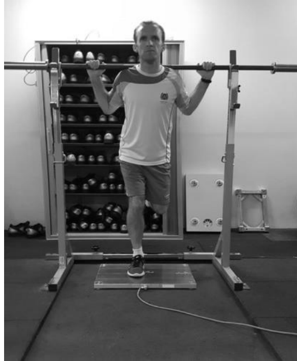
Figure 2: Adopted subject positioning for the unilateral isometric strength test. Squat rack was bolted to the floor, and had custom made stoppers connecting the barbell to the rack.
