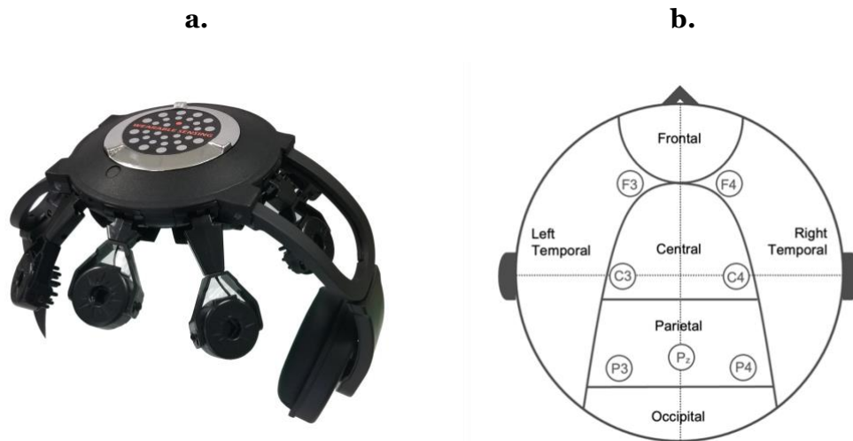
Figure 1: Displays the: a) dry-electrode EEG system (DSI-7, Wearable Sensing, LLC, San Diego CA) and b) the electrode placement used, with electrodes (F3, F4, C3, C4, Pz, P3, P4) based upon the International 10-20 system.
