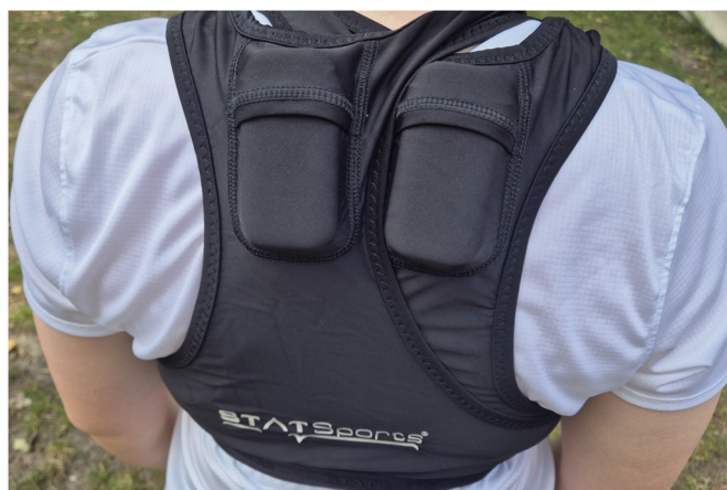
Figure 1. STATSports Apex Pro GNSS unit alignment in harnesses on the upper-back for assessment of interunit reliability.
